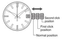
For models with a screw down crown, remember to screw the crown in.
