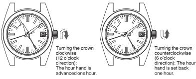
\* The crown can be turned in either direction to set the date, however, it is recommended to turn the crown in the direction which enables you to set the time difference with a smaller adjustment.
