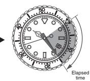
Read the graduation on the rotating bezel to which the minute hand is pointing.
