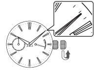
③ Turn the crown clockwise (12 o'clock direction) to return the minute hand to the desired time.
